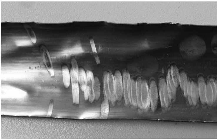
Figure 4. Peeled-off surface of a zircaloy hull by laser.
